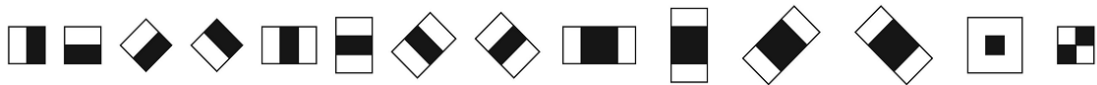
FIGURE 2.1: Haar wavelets. Black and white areas denote negative and positive weights, respectively [6].
