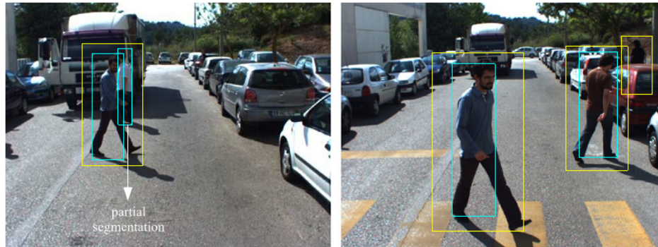
FIGURE 3.8: Two scenarios where traditional laser and vision fusion systems could fail. The light bounding box (yellow) is the result of an image classifier; the darker ones (blue) are the result of laser segmentation. [15].
