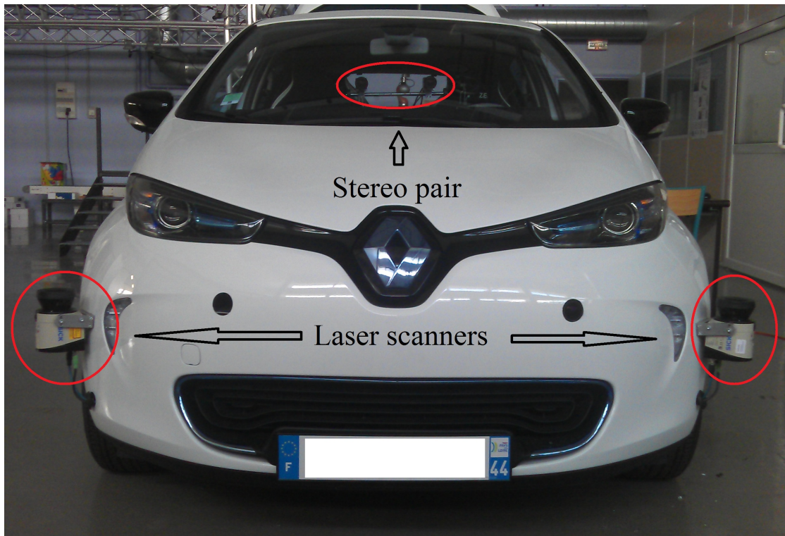
FIGURE 1.4: Renault ZOE equipped for pedestrian detection and tracking.
